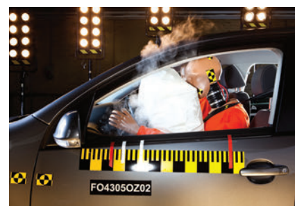
▲ Figure 3.6 Decomposition of sodium azide, \text{NaN}_3(s) , produces \text{N}_2(g) that inflates air bags in automobiles.
