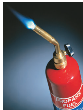
▲ Figure 3.7 Propane burning in air. Liquid propane in the tank, \text{C}_3\text{H}_8 , vaporizes and mixes with air as it escapes through the nozzle. The combustion reaction of \text{C}_3\text{H}_8 and \text{O}_2 produces a blue flame.
