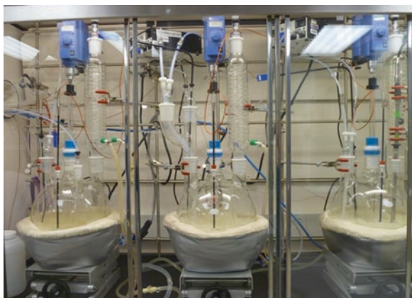
Fig. 2.12 Picture of three 12 L CSTRs-in-series used for a continuous Schotten-Baumann reaction
