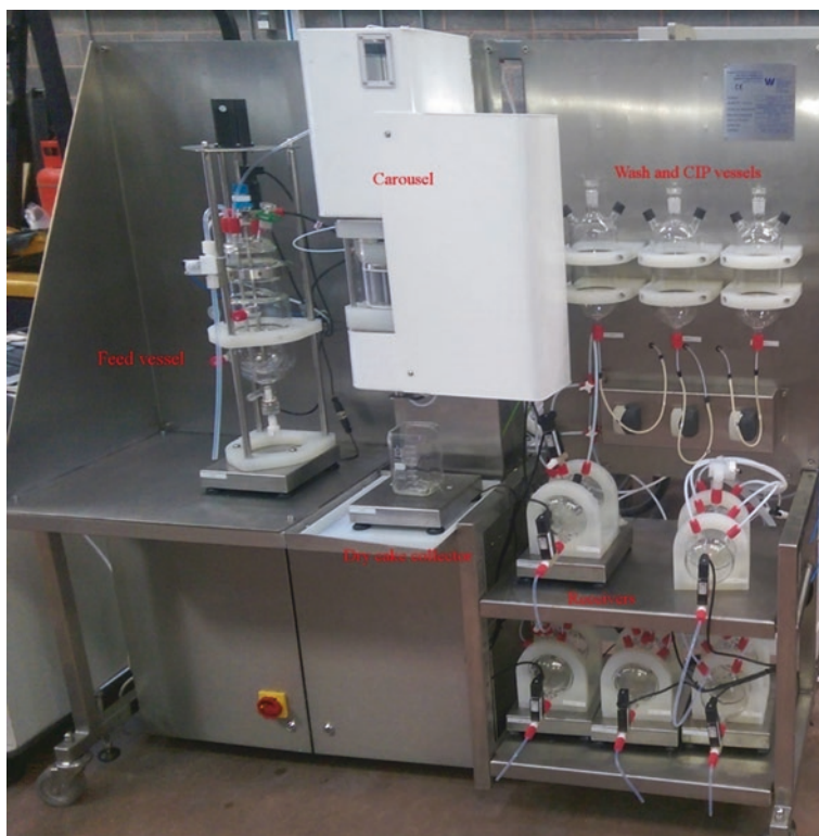
Fig. 5.45 A continuous filtration drying unit developed by AVL. (Permission obtained from Ottoboni et al. © 2019 American Pharmacists Association®. Published by Elsevier Inc.)
