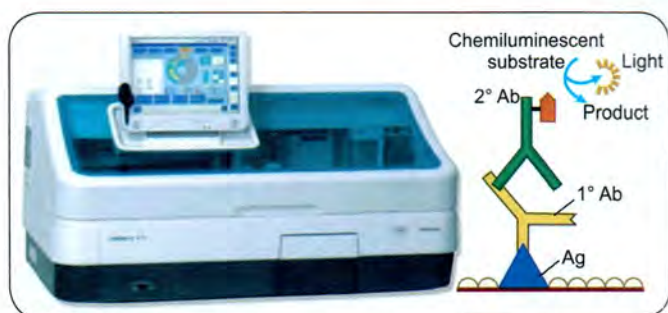
Fig. 12.22: Chemiluminescence system (CLIA) and its principle
